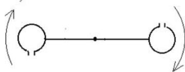
Figure 10.13: Two identical resonators (viewed in a horizontal plane) hung from a thin wire connected to the center of the cross bar, as shown. A sufficiently strong sound wave at the resonance frequency of the resonators will make the resonators move, as indicated, so that the resonator assembly will rotate about its vertical axis of suspension.
